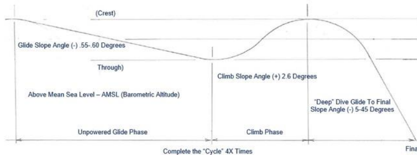
LOCOST Pulse Gliding Flight Profile Example For JFIX
