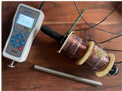
Figure 1 shows a functioning Sektet engine which produced a maximum of 8.65 N net force. The engine consists of two solenoid coils, connected to two separate power supplies and a 99.7% pure iron momentum and magnetic conductor.
