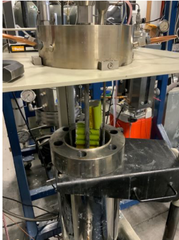
Lithium cells from a BB2590 being deactivated at OnTo Technology LLC facility in Bend, OR.
