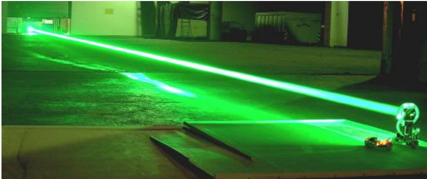
EADS Astrium tracking laser to power rover (2003)
