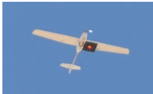
LaserMotive outdoor laser power to UAV (2012)
