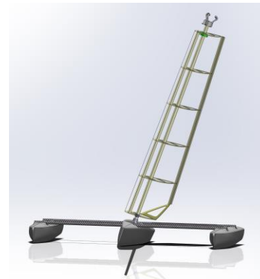
HERMES with rolled rig in response to heeling moment
