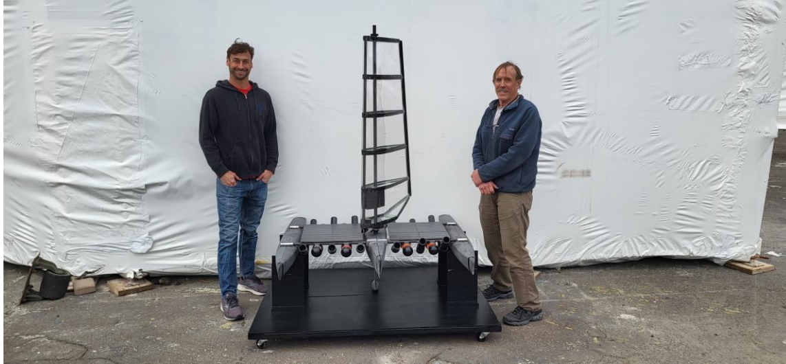
Left: SSS partners with 4'x4' prototype. Self righting from any possible capsizing. Note keel & flotation in wing.
