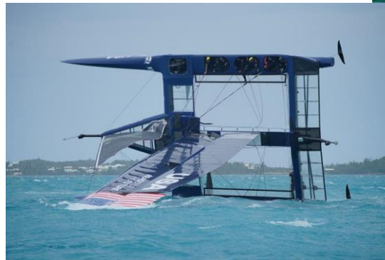
Right/below: Traditional capsizing risk for multi-hull vessels limits their usage.
