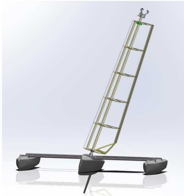
Left: HERMES with rolled rig in response to heeling moment increased resistance to capsizing
