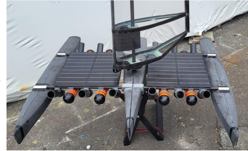
Right: HERMES deck showing solar panels + tube launched possibilities.
