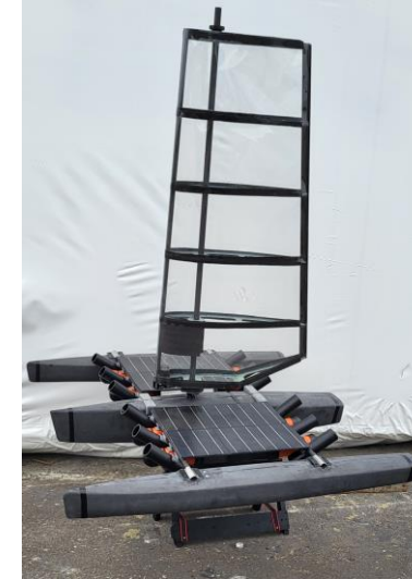
HERMES with rolled rig in response to heeling moment
